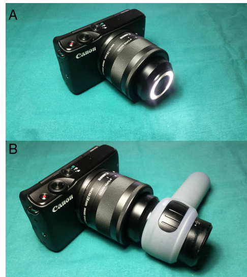
Figure 1 Canon EF-M 28 mm F3.5 Macro IS STM lens. A, Notice the light emitting diode system on the front of the lens. B, The lens is easy to attach to a dermoscope.
