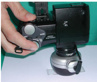
Figure 3. Position of camera, dermatoscope, and microscope slide to obtain the panoramic image.
